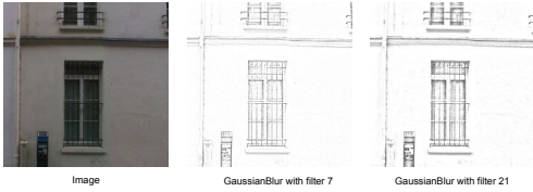
Figure 4: Illustration showing the degree of structural and texture information that can be recovered by using a larger or smaller Gaussian filter.
