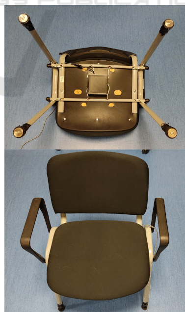
Figure 2: Actual images of the prototype: the four compression load cells are the only contact points with the floor.
