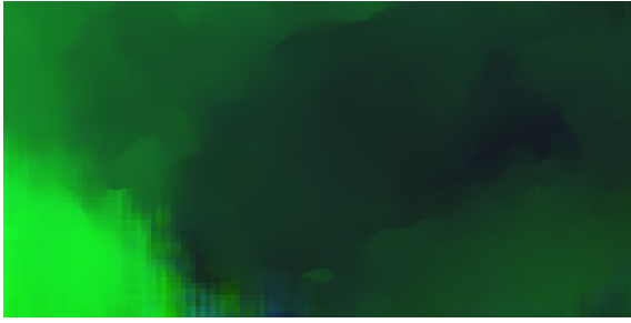
Figure 6: The disparity map of the case shown in Fig. 5. Dark pixels refer to regions far away from the camera and bright pixels refer to regions closer to the camera. The white area on the left holds no information due to the stereoscopic baseline shift. In addition, due to the baseline shift and missing information, there is also an incorrect prediction of a region distant from the camera system (red pixels) that is actually close to the camera system.
