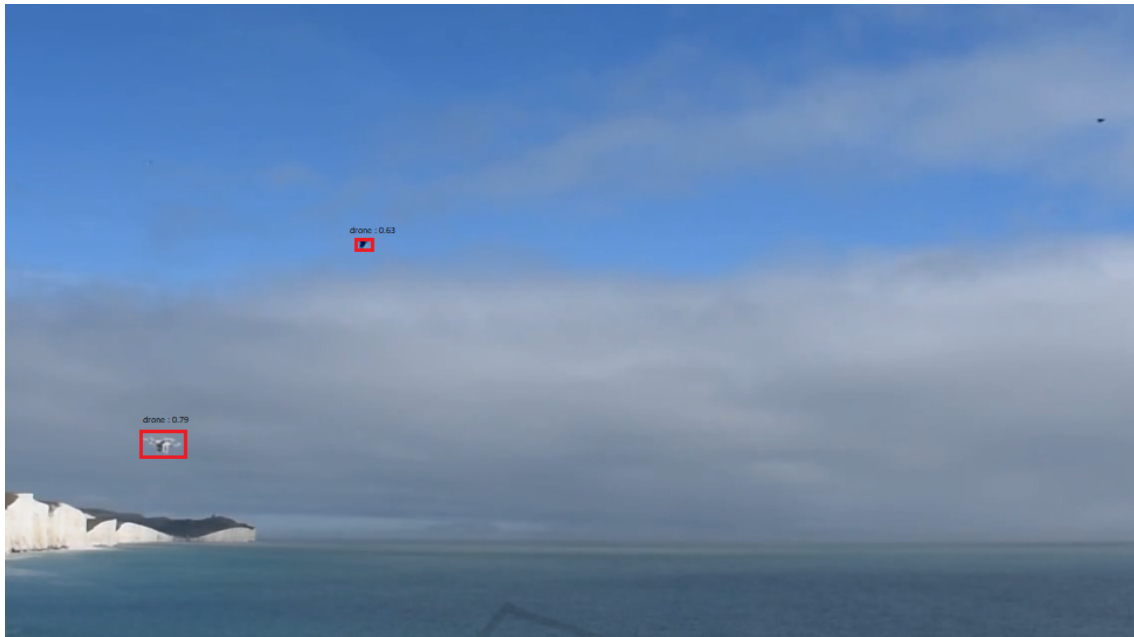
Figure 1: YOLO output shows how it detects bird(on top) as a drone thus giving a false positive in a video from the Drone vs. Bird dataset.
