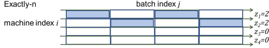
Figure 3: General assignments ( Exactly-n and Exactly-n Ordered ) for an example with n = 4 batches (columns) on m = 4 machines (rows) with z_1 = z_2 = 2 , z_3 = z_4 = 0 .
