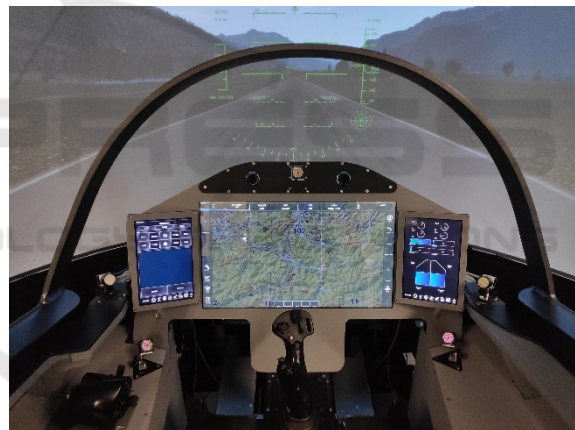
Figure 1: Jet simulator cockpit at the HuMiCS Lab. Setup consists of a throttle, stick, three touch display and a projected outside view with a head-up display overlay.
