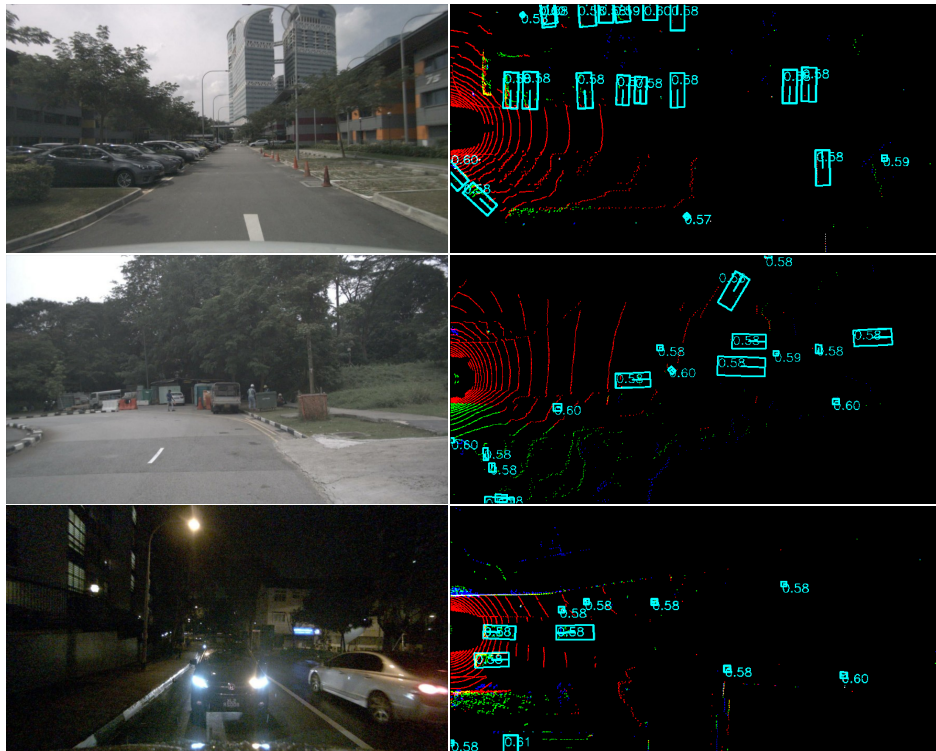
Figure 5: Visualization of the BEV detections predicted by our model. The model has good prediction for most cars, but has difficulties at the edges of the BEV lidar. It cannot detect all construction workers in image two, however construction workers are underrepresented in the dataset. At night the detection of the cars is very good despite the low visibility.
