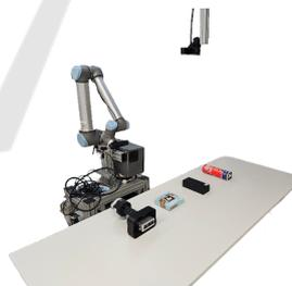
Figure 3: Real setup consisting of UR10e robot, overhead mounted camera, and tabletop objects.
