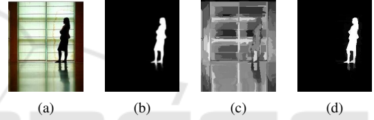
Figure 4: Image with complex background with little relevant information from background queries. (a) original image; (b) U2Net map; (c) background-based saliency with d_{0.5} < 0.1 ; (d) background-based saliency from last iteration which will substitute (c).
