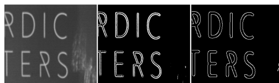
Figure 3: Cropped images: (left) image without filter, (middle) image with Sobel, and (right) image with Canny. Reflections and the luminous background are reduced by applying these filters.
