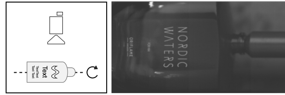
Figure 2: Photography setup: (left) system overview and (right) a captured image. The camera and lighting remain stationary during the capture, and the bottle is rotated.
