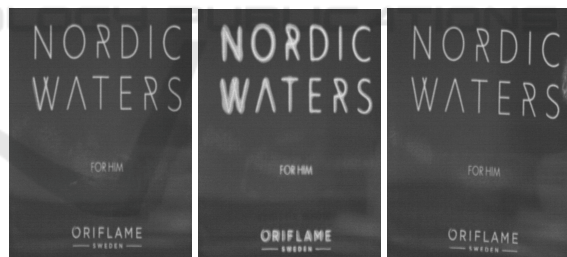
Figure 1: Cropped images of glass bottle prints: (left) acceptable print, (middle) unacceptable smeared print, and (right) unacceptable rotated print.
