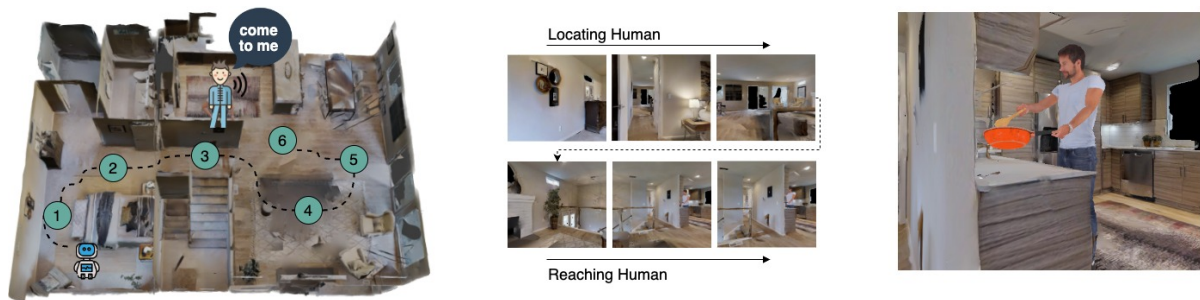
Figure 2: (Left) Robot responding to a human call by exploring the environment with the help of multiple global goals (1-6) to locate and reach the human. (center) Robot’s observations upon reaching each global goal (1-6) during its exploration of the environment. (right) Robot’s final observation upon successfully reaching the human at an appropriate angle, depending on the human’s activity, to initiate a conversation.
