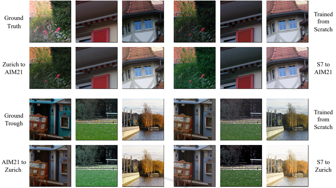
Figure 5: Predictions visualization for Domain adaptation from source domains to Zurich RAW-to-RGB and Mobile AIM21. Training from scratch – an AW-Net ISP pipeline trained from scratch on the corresponding dataset (Mobile AIM21 on top, Zurich RAW-to-RGB on bottom). Zurich to AIM21, AIM21 to Zurich, etc. – a demonstration of the work of our domain adaptation approach on 10 images for the corresponding datasets.
