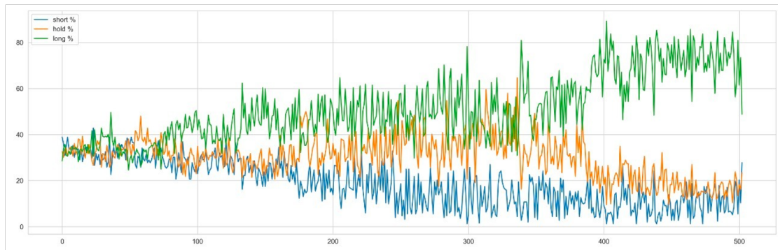
Figure 8: During the first 200 episodes, the agent is designed to explore the environment by choosing random actions, so the distribution for each action is close to 33%. As the training progresses, it slowly shifts to a more stable strategy, choosing mainly long actions as a safety net, while short actions are rarely chosen. This diagram can be used as evidence that our agent is learning and not sticking to a usual trading strategy like buy and hold.
