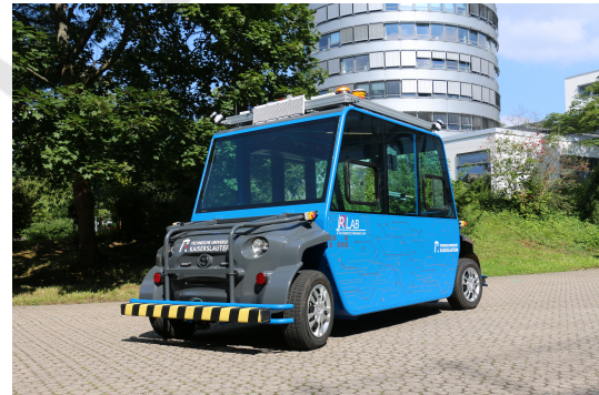
Figure 1: Driverless Minibus on campus of RPTU Kaiserslautern-Landau (Jan and Berns, 2021). It is meant to ferry 6-8 people from building to building in the campus.
