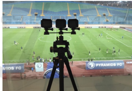
Figure 2: Camera setup for panoramic view creation.
