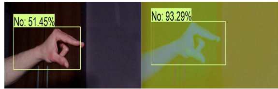
Figure 6: Sign recognition comparison between RGB and YCbCr color spaces in low-light environment. YCbCr outperforms RGB in this condition.
