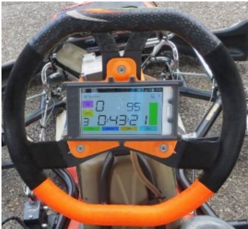
Figure 4: Driver monitor mounted over the steer to immediate view of some driving parameters.
