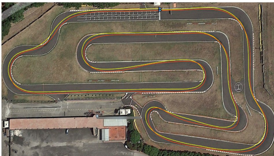
Figure 10: Trajectories recorded by the system differentiate between those acquired with RTK correction (in red) and those obtained without it (in yellow).
