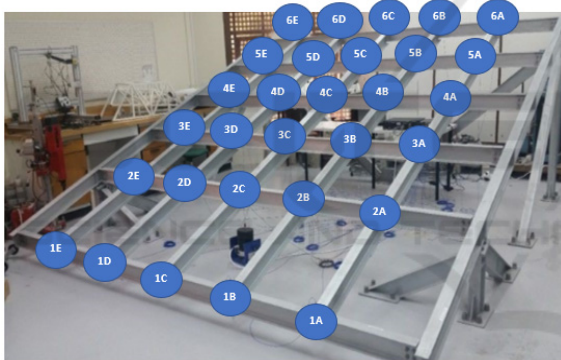
Figure 3: QUGS Sensor Point Locations Identified. Source: Adapted from (Abdeljaber et al, 2017).
