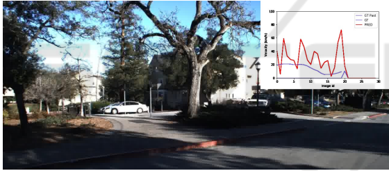
Figure 8: Wrong ego-vehicle speed predictions (from the CNN+LSTM model) when the ego-vehicle data is corrupt/erroneous.
