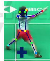
Figure 4: Acquisition of skeletal information and player position. Blue crosses is the midpoint of both ankles and defined as the player position.
