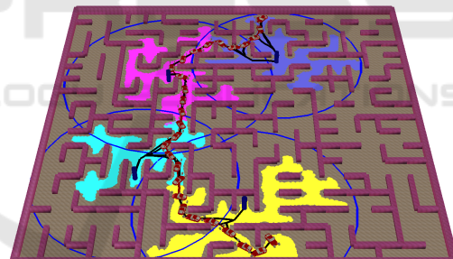
Figure 1: Example of path planning with safety zones for a car robot model. Each safety zone is defined by its center (blue cylinder) and radius (blue circle). For each intermediate configuration along the main path to the goal, the figure also shows the emergency route (black segments) to reach a safety center within the distance constraints. If an emergency path partially overlaps with the main path, only the non-overlapping portion is visible. The safe locations (from which a safety center can be reached within the distance constraints) are shown in yellow, cyan, magenta, and blue for safety zones 1, 2, 3, and 4, respectively. Videos can be found at https://tinyurl.com/y4d2urcf .
