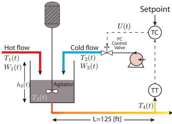
Figure 1: Mixing Tank process.
