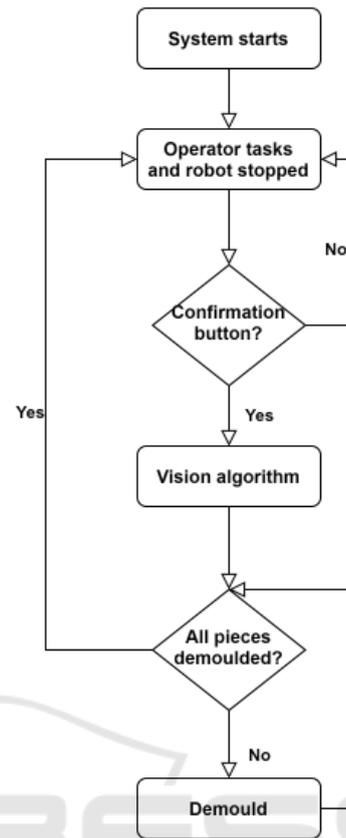
Figure 6: Automatic demoulding pipeline.
