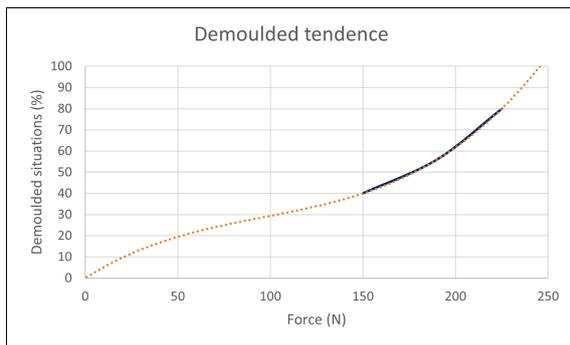
Figure 13: Trend of Demoulded situations as a function of the force applied by the robot.
