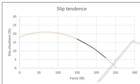
Figure 10: Trend of slip situations as a function of the force applied by the robot.
