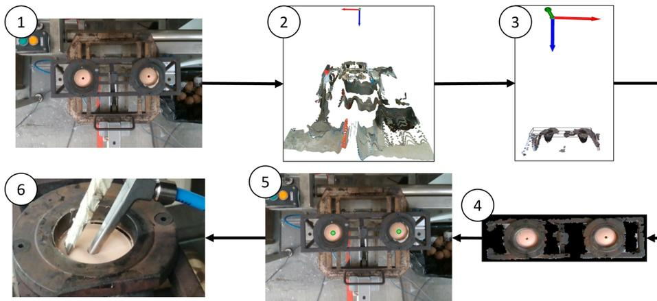
Figure 8: Vision-based algorithm process for extraction point detection.
