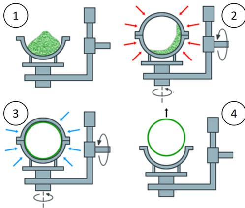
Figure 1: Rotomoulding manufacturing process.
