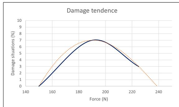
Figure 11: Trend of Damage situations as a function of the force applied by the robot.
