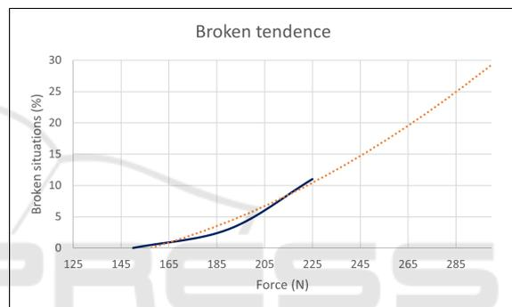
Figure 12: Trend of Break situations as a function of the force applied by the robot.
