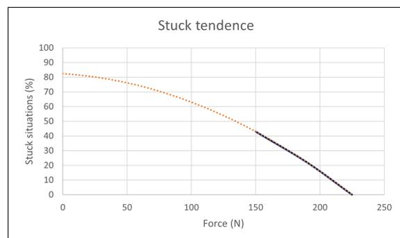
Figure 9: Trend of stuck situations as a function of the force applied by the robot.
