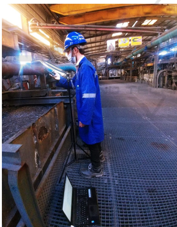
Figure 3: The data acquisition system of the flotation froth videos.
