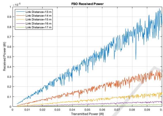
Figure 2: The power on the receiver side, with a visibility of 10 km and for different TX and distance values.
