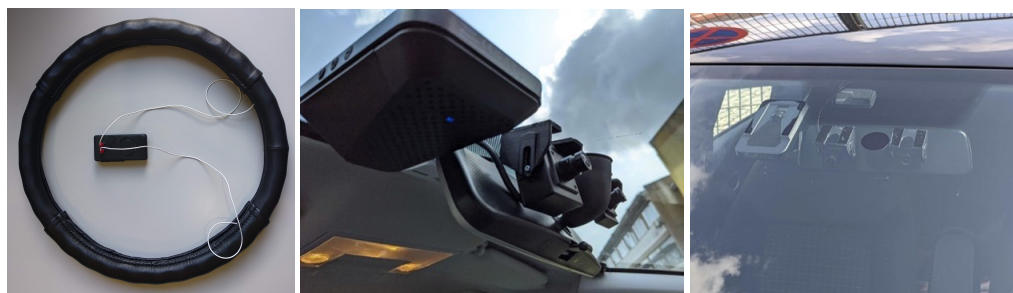
Figure 2: CardioWheel on the steering wheel (left). Mobileye and dashcam seen from the inside (middle) and from the outside of the vehicle (right).
