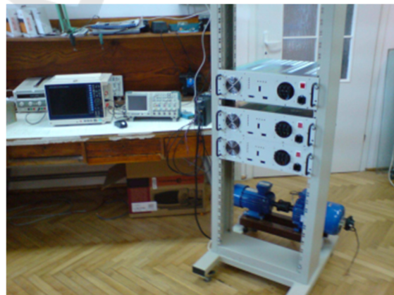
Figure 12: The simulator with connected measurements and data acquisition instrumentation.
