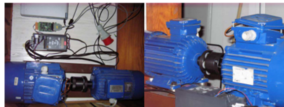
Figure 10: Ga Turbine set hardware-based model with an inverter drive by Danfoss.
