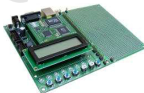
Figure 8: A view of motherboard which integrating a microcontroller ATMEGA 128 16 MHz with Ethernet controller RTL1819AS IEEE 802.3 10Mb/s for carrying out the function of a web server.
