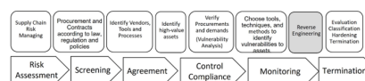
Figure 2: Proposed inclusion of a Reverse Engineering subprocess into the equipment procurement process at a DSO.
