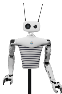
Figure 3: Rechy’s Full kit picture: 3D printed MJF Painted - Flexible PU molded - Aluminium Construction; 670x1800x200mm with arms outstretched; 180 W of Max Power consumption and 6.2 kg of weight.
