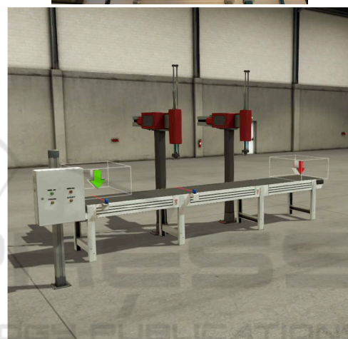
Figure 9: Station 3 of the FESTO plant (up) and its Factory I/O model (down).
