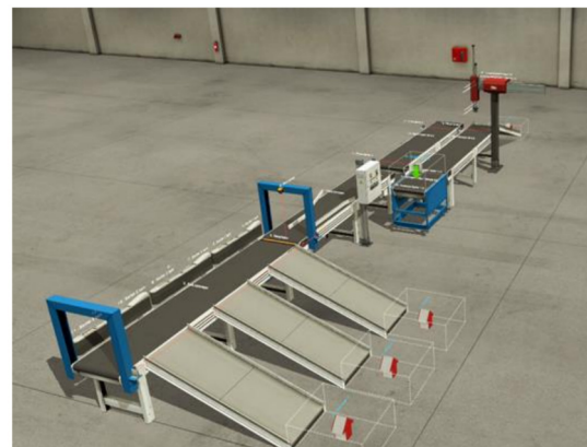
Figure 5: Automation of a box weighing and colour sorting system.
