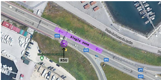
Figure 5: Single tolling scenario used for the first road trial.
