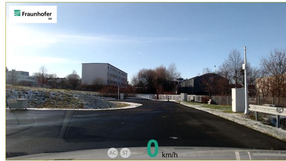
Figure 3: Screen shot of the remote driving desktop, showing the video stream from the vehicle as well as current velocity and the status of the acceleration (AC) and steering (ST) interfaces. The gray color indicates deactivated interfaces, i.e., no remote driving is possible at the moment.
