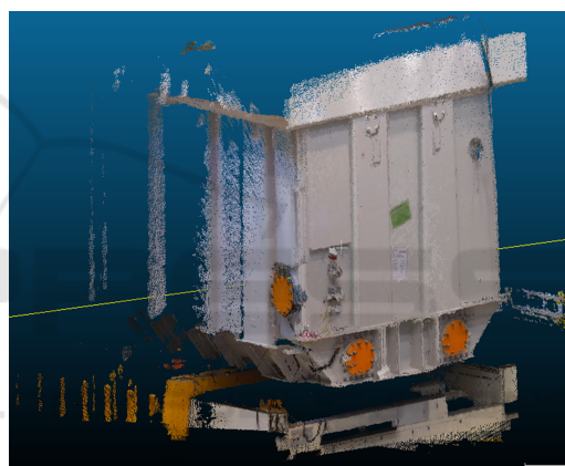
Figure 4: View on a transformer with an RGB-D sensor (Microsoft Azure Kinect).
