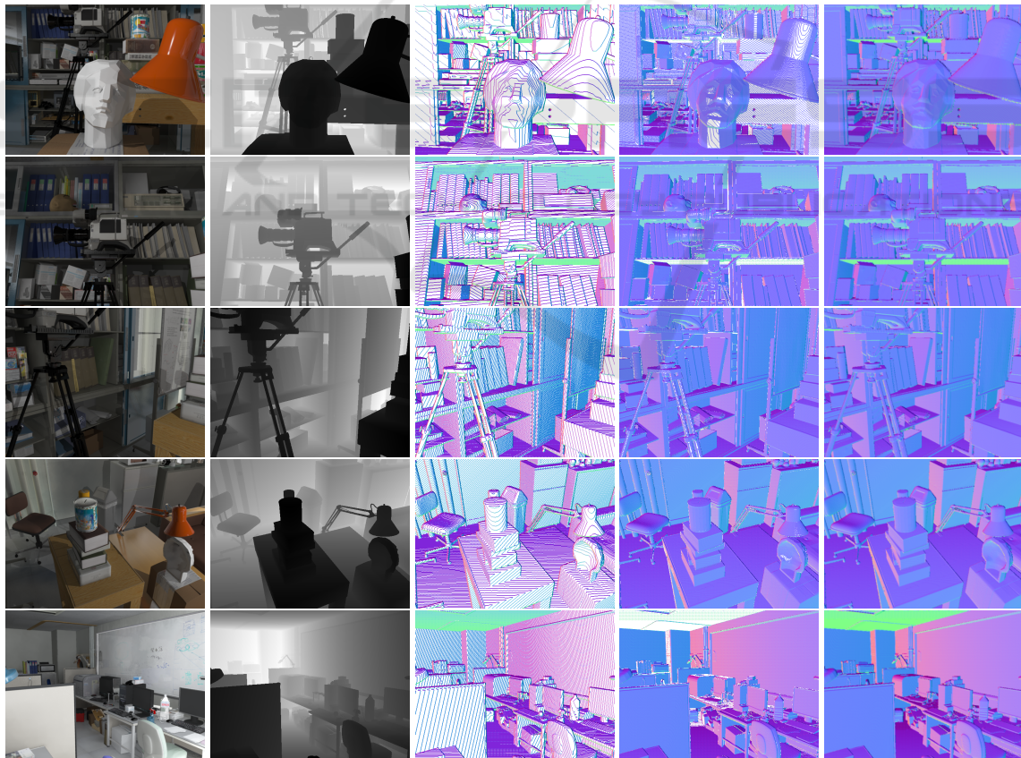
Figure 9: Visual comparison on the New Tsukuba Dataset. (Left-to-right) The scene, depth map, and estimations of Angle-Weighted, proposed without scale-space and proposed with scale-space. The white regions present the pixels, where surface normals could not be computed. Note here that a different threshold is used according to the range of this dataset.
