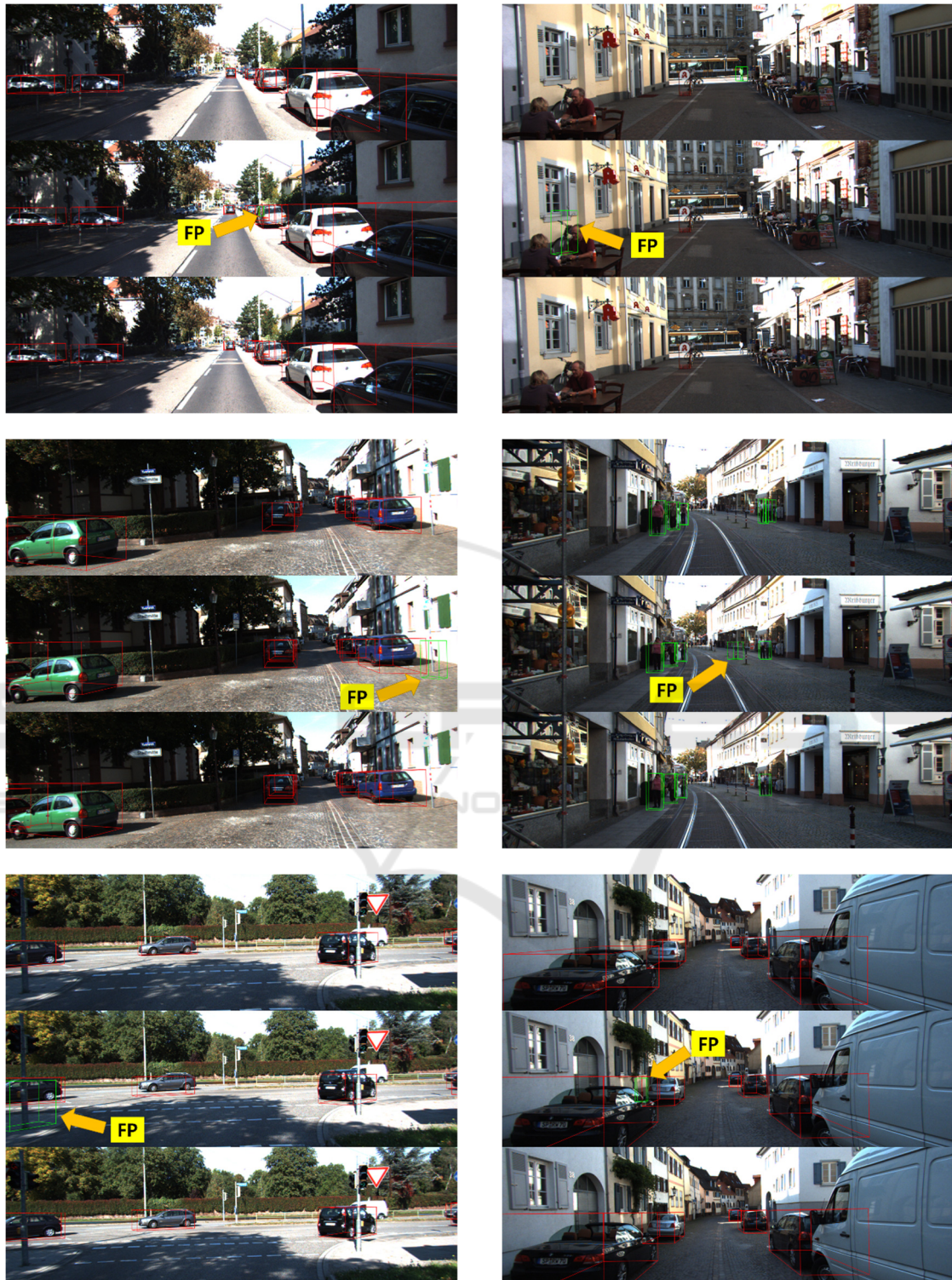
Figure 10: Improvement performance of the proposed method that uses the shape loss function with reduced false positive errors (top: ground truth, middle: outputs of the complex YOLO algorithm, bottom: proposed method).
