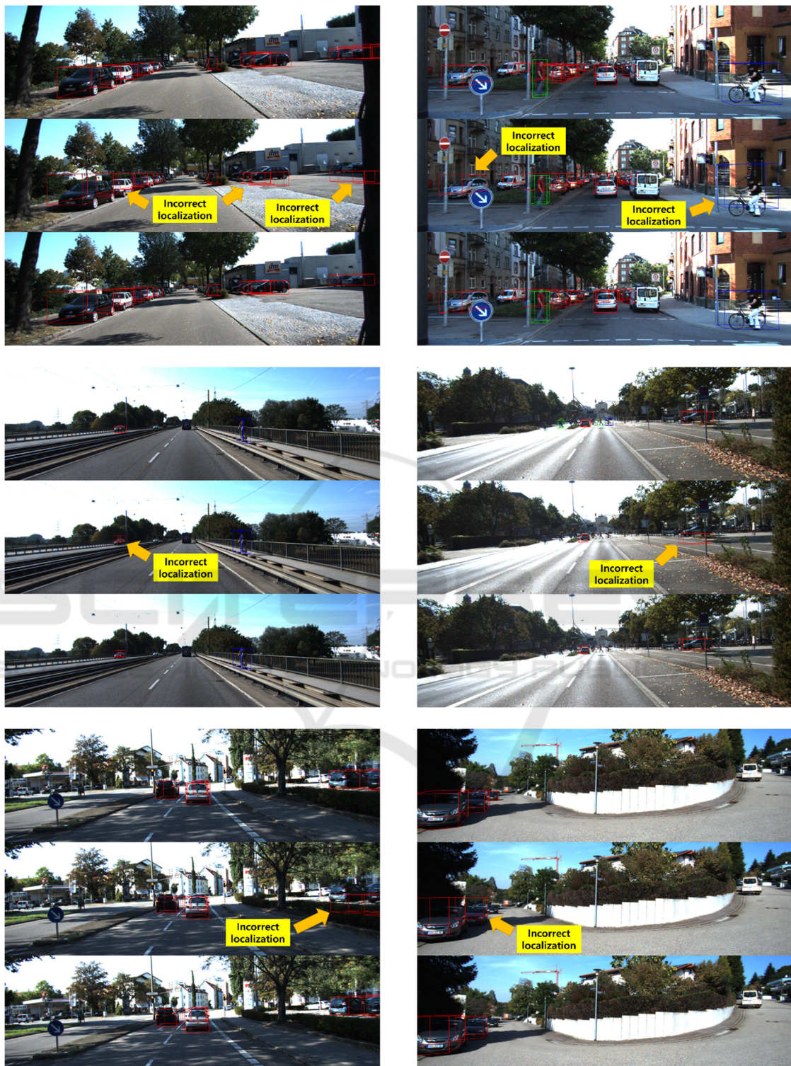
Figure 9: Improved localization (ground ROI estimation) of the proposed adaptive ground ROI estimation method (top: ground truth, middle: outputs of the complex YOLO algorithm, bottom: improved ground ROI estimation of the proposed adaptive ground ROI estimation method).
