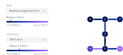
Figure 2: The undirected graph of the qubits for the ibm_oslo quantum computer (IBM Quantum, 2022h).
