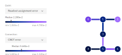
Figure 1: The undirected graph of the qubits for the ibm_nairobi quantum computer (IBM Quantum, 2022g).
