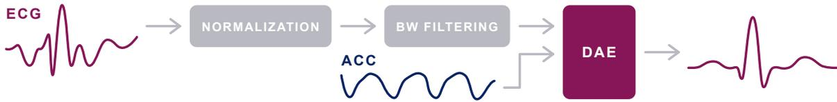
Figure 3: Proposed ECG denoising pipeline. Inputs: Noisy ECG and correspondent ACC. Output: Denoised ECG estimate.
