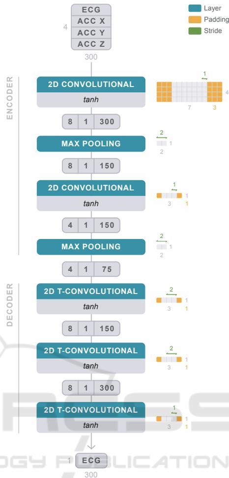
Figure 4: Proposed DAE architecture. Kernel sizes on the right side of each layer. Tensor sizes in (C, H, W) format.
