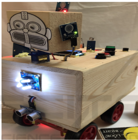
Figure 6: Front view of Kodockly 2.0(Mohamed et al., 2021).
