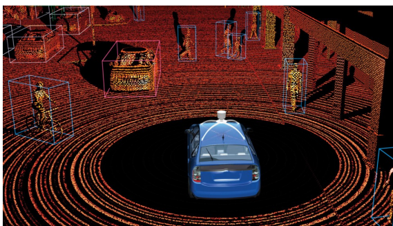
Figure 1: An image of an autonomous car using LiDAR as distance measure and camera as object detection (Cameron, 2017).
