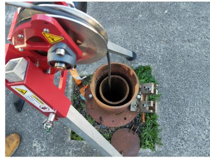
Figure 3: Winch used to send detector down into the test borehole.
