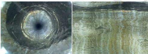
Figure 5: Original frame and corresponding unwrapped side view image.
