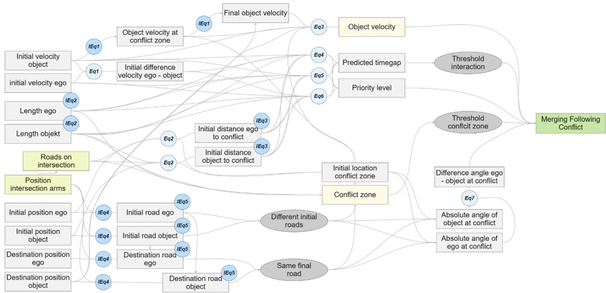
Figure 5: Hybrid graph of a merging following conflict including observed parameters (yellow), unobserved parameters (light yellow), infrastructure parameters (green), equations (Eq), inequalities (IEq) and thresholds (gray).
