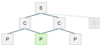
Figure 4: Combined graph with scenario (S), concepts (C), and their parameters (P) for generation of detailed scenarios.
