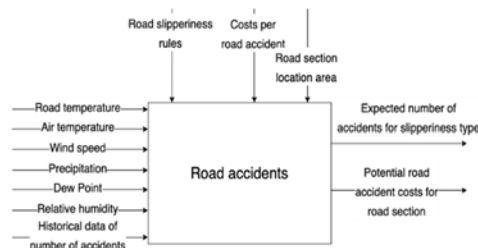
Figure 3: Inputs and outputs calculating potential road accident costs and expected number of slipperiness type.
