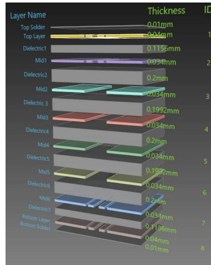
Figure 3: Defined ECU PCB layer stackup from a design tool.
