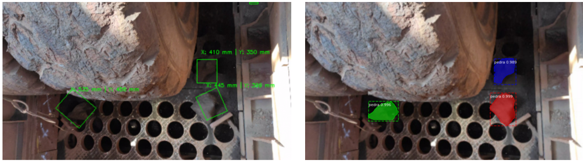
(a) Detection performed by Souza (Souza, 2020) using U-Net (b) Detection performed by Mask R-CNN with ResNet101
