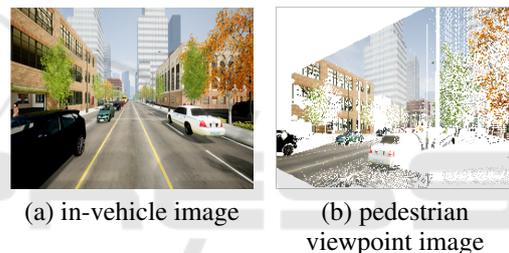
Figure 1: Viewpoint transfer with depth estimation. The viewpoint-transformed image in (b) contains a large amount of missing regions that are not visible in the original camera image in (a).
