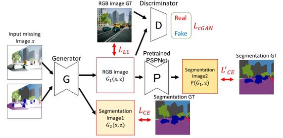
Figure 3: Network structure of method 2. We evaluate the quality of complemented RGB images by combining semantic loss with adversarial loss to further improve the performance of the generator.
