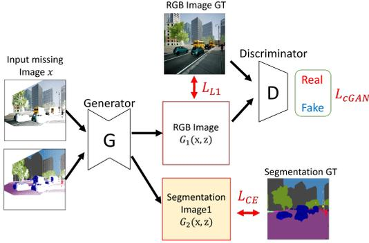
Figure 2: Network structure of method 1. Generator receives missing RGB images and missing label images, and outputs generated RGB images that complement missing RGB images and generated label images that complement missing label images.
