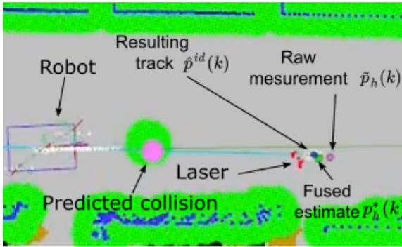
Figure 4: Camera and laser data fusion for improved human pose estimation. The laser data points (red points), the raw measurement  $\tilde{p}_h(k)$  from the human detection (purple), the measurement from the fused estimate  $p_h^*(k)$  (green) and the resulting track influenced by the Kalman filter  $\hat{p}^{id}(k)$  (blue).
