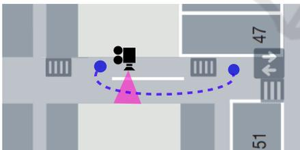
Figure 6: The test setup: The purple area represent the field of view of the camera for people counting; the dashed line suggest a possible path for the robot from start to end point.
