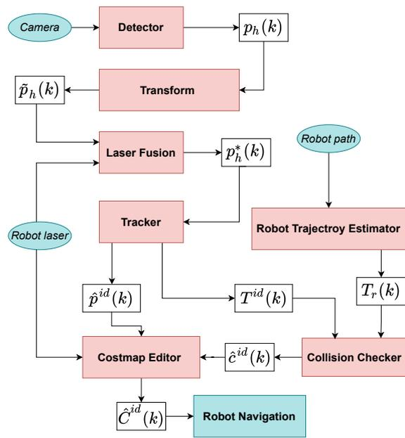
Figure 2: System overview - components colored in blue are part of the mobile robot navigation stack, components colored in red are introduced in the proposed solution.
