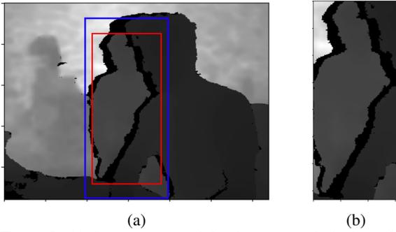
Figure 3: A) shows a captured depth image with the bounding box (blue) for the detected human and the downscaled bounding box (red). B) shows the cropped image used for human position estimation.
