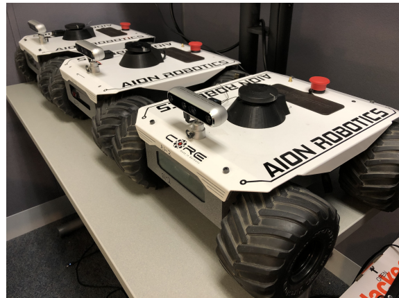
Figure 3: Three rovers used in the MAAP capstone. In addition to the standard RC radio, autopilot, and GPS systems, we attached an Intel® RealSense™ D455 depth-sensing camera.
