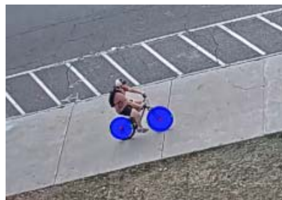
Figure 8: Detection of bicycle wheel using Hough Transform.
