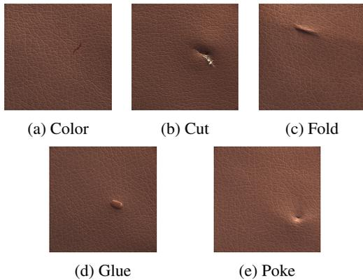
Figure 1: MVTEC leather defect samples.
