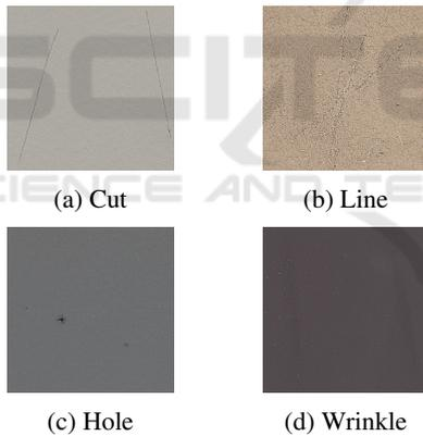
Figure 2: Neadvantage leather defect samples.
