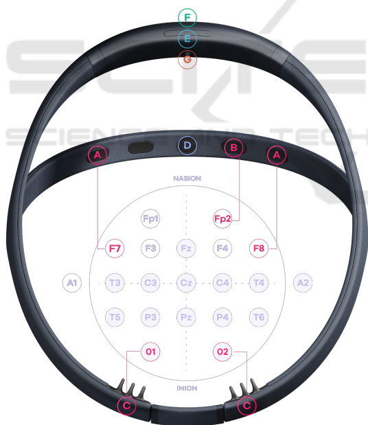
Figure 2: Electrode placement for Dreem EEG sensor.
